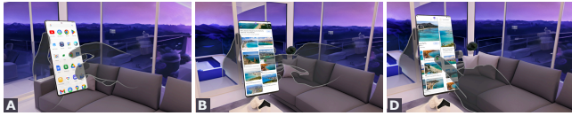
Figure 10: Navigating a web browser with a Phone-Locked and Touch interactive smartphone. Looking for vacation inspiration in Hawaii, A) the user navigates to the web browser via target acquisition, B) browses images through pictures with scrolling, and C) navigates pages through swipes.
